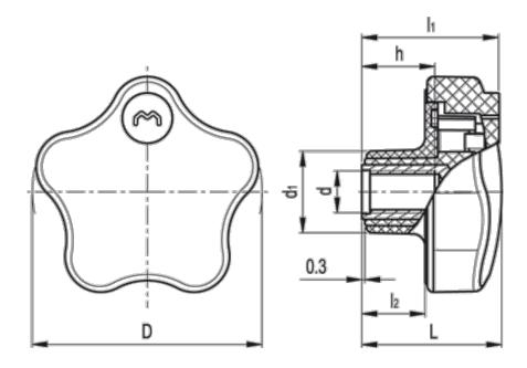
D = 41.5 d1 = 16.5 d 6H = M6 h = 12 L = 30 l1 = 29.5 l2 = 14.5 Weight (g) = 25
